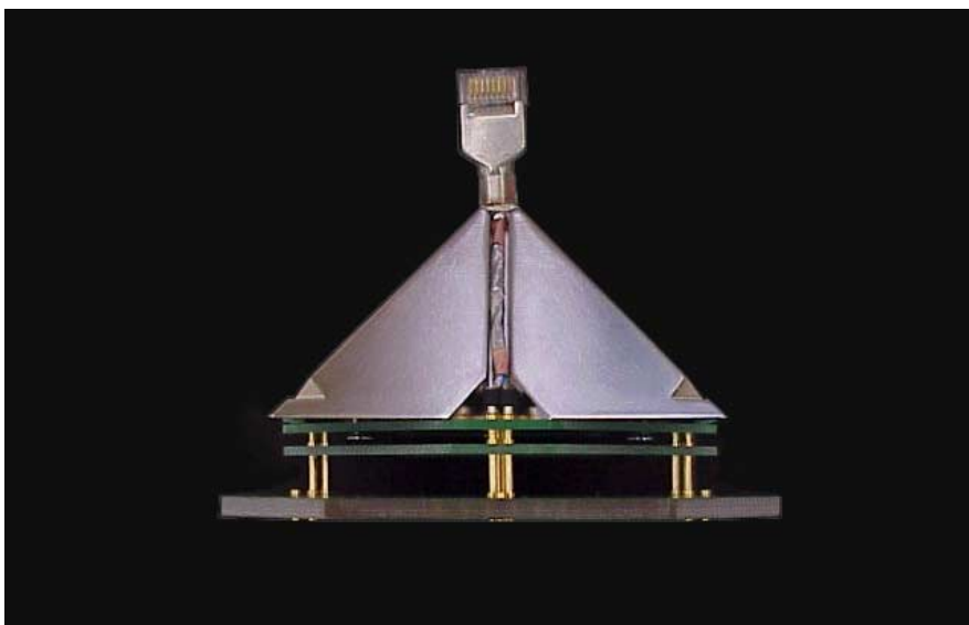
De-Embedded Test Set Up (ANSI/TIA/EIA-568-B.2 SP-3737-AD1-B)
